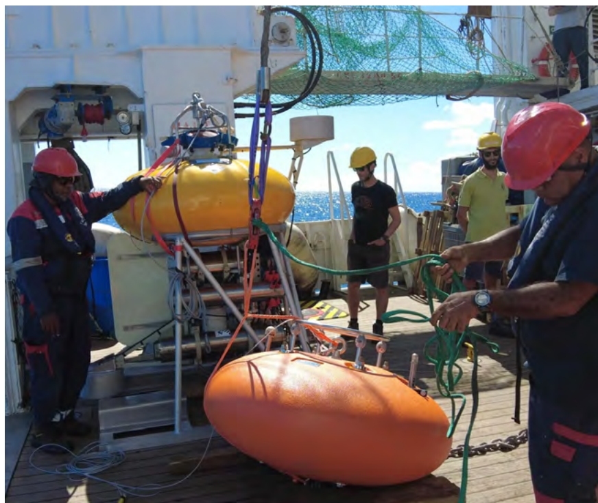
Deployment, from R/V Antéa , of an experimental mooring line fitted with sensors and sampling equipment to observe the little-known and biodiversity-rich ecosystems of Coral Sea seamounts near New Caledonia.
